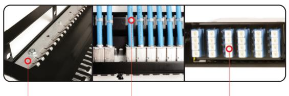
Installer Friendly – Panels feature an integrated grounding strip to ensure proper ground path from copper outlets to grounding point Cable Management – Built in cable manager provides ability to secures cables for proper strain relief Plug & Play – Panels utilize the Plug & Play adapter modules that utilize NY-LATCH (push-pull adapters) for ease of installation
